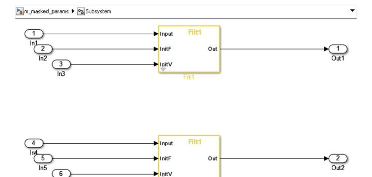
The two subsystems, Filt1, and Filt2, have different values assigned to their mask parameters. In this example, Filt1\_Order\_Thau is a constant with a value of 5.
