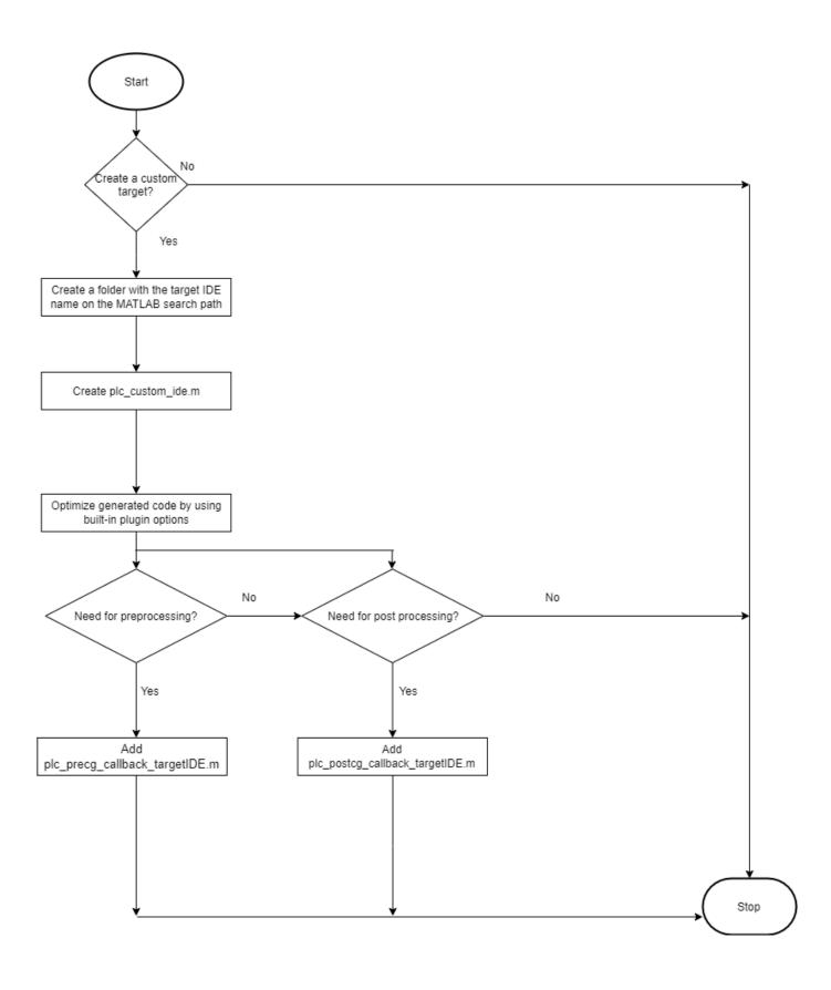
Follow the flowchart to create the plc\_custom\_ide.m and if required the plc\_precg\_callback\_IDEname.m, and plc\_postcg\_callback\_IDEname.m files. To use these files to create and generate code for your custom target IDE, see "Generate Code by Using Plugin-Based Target IDE" on page 29-15.
