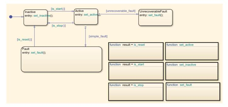
The ControlModule chart performs the drive control logic.
