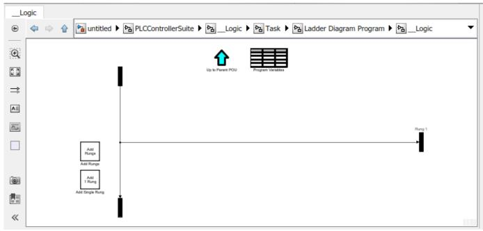
Use the XIC and OTE blocks from the library to construct a simple ladder diagram. Use the **Add Rungs** or **Add 1 Rung** buttons in the ladder logic semantic to add a new rung. All added blocks must be on the rung. Use the Junction block to merge rung branches.
