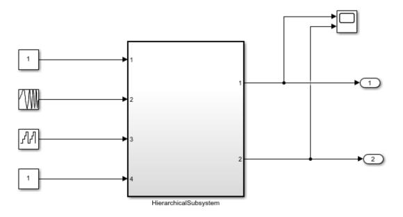
This introductory model shows the code generated for a hierarchical subsystem consisting of two other subsystems named "S1" and "S2". Each of these subsystems generate a separate Function Block. To build the subsystem, right-click on the subsystem block and select PLC Code > Generate Code for Subsystem.
