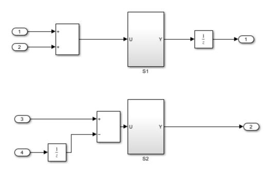
You can generate PLC Structured Text code for this subsystem by right-clicking on the subsystem block and select PLC Code -> Generate Code for Subsystem Alternatively, you can use the following command
