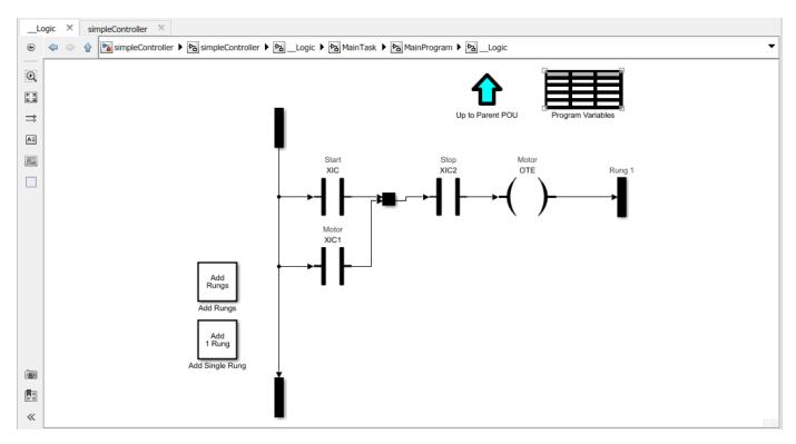
To generate C code for the subsystem simpleController/simpleController, you must first enable the 'FastSim' option for the Simulink Ladder Diagram model.
