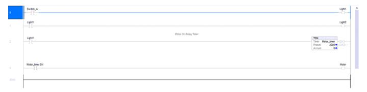
Light1, Light2, and Motor are the outputs of this ladder diagram.
