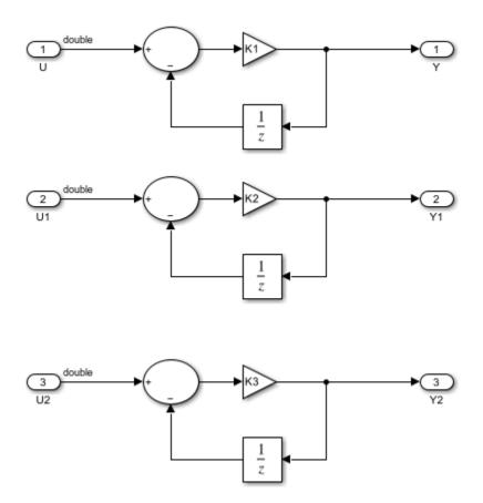
This model shows the different implementations of tunable parameters in the generated code. It makes use of three parameters K1, K2, and K3 defined in the MATLAB base workspace. To build the subsystem, right-click on the subsystem block and select PLC Code Generation > Generate Code for Subsystem. The Diagnostic Viewer with hyperlinks to the generated code is displayed automatically.
