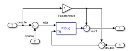
You can generate PLC Structured Text code for this subsystem by right-clicking on the subsystem block and select PLC Code -> Generate Code for Subsystem Alternatively, you can use the following command
