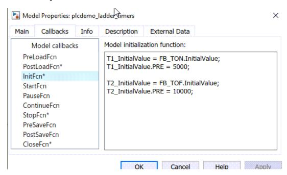
To specify a preset delay, enter the value in milliseconds into the TimerName\_InitialValue.PRE. For example, T1\_InitialValue.PRE is set to 5000, which means a time delay of 5 seconds and T2\_InitialValue.PRE is set to 10,000, which means a time delay of 10 seconds. You can simulate different start and stop delays by changing these timer presets to different values.
