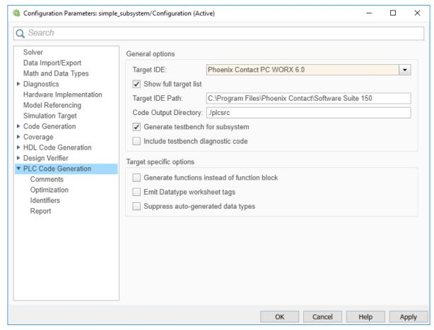
On the **PLC Code Generation** pane, select an option from the **Target IDE** list, for example, 3S CoDeSys 2.3.
