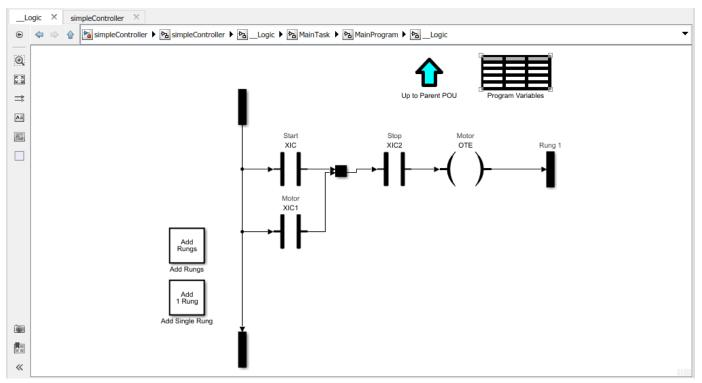
**6** Double-click each new block added to the rung and specify the tags. In ladder diagrams, tags (variables) represent all inputs, outputs, and internal memory. The tag can be a variable name or an expression, such as:
