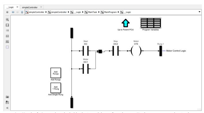
**9** Use Ctrl+D to update the ladder logic model to reflect changes. You have now created a simple ladder model in Simulink.
