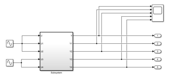
This model shows the use of Simulink Data Dictionary to specify model parameter and signal data and generate PLC code. The parameters K1, K2, K3, and signals dsm1, dsm2 are defined in data dictionary file plc\_sldd\_ex.sldd. To generate PLC code, open PLC Coder App. Select the Subsystem block and click the Generate PLC Code button.
