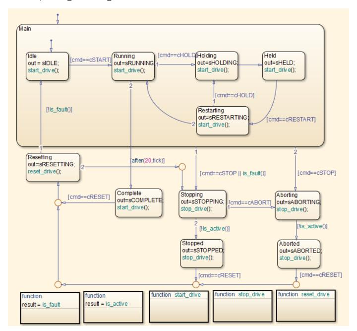
You can map the states and transitions in the chart to the generated code. For instance, the transition from the state Aborting to Aborted appears in the generated code as:
