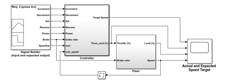
This model shows PLC code generation using variable-step continuous solver for a Speed Cruise Control controller subsystem. PLC Coder supports code generation of model controller subsystem block with fixed sample time. To satisfy this requirement, user can
