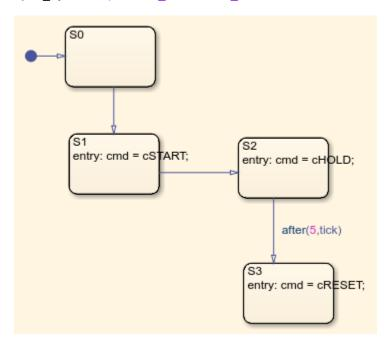
The BehaviorModel chart provides a simple chart to test the ControlModule chart behavior by injecting faults.
