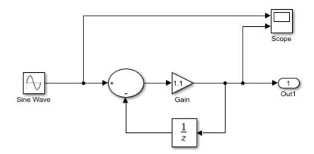
Configure the model to use the fixed-step discrete solver. Click the solver link in the lower-right corner of the model window. In the Solver information pane, click View solver settings to open the Solver pane of the model configuration parameters. Under the Solver selection, set Type to Fixed-step and Solver to discrete (no continuous states).
