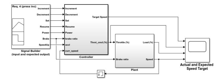
This model shows the code generation for the Speed Cruise Control Controller subsystem. Open the Controller subsystem. This model uses a Triggered Stateflow Chart for the Enable and Setpoint calculations. It uses a discrete PID Controller to compute the Throttle Command. Click the scopes to observe the Target and Actual speeds.
