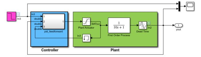
This model shows the code generated for a PID Feedforward Controller subsystem.
