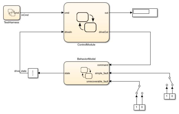
This example shows the use of a Stateflow chart to implement the control logic for a drive.
